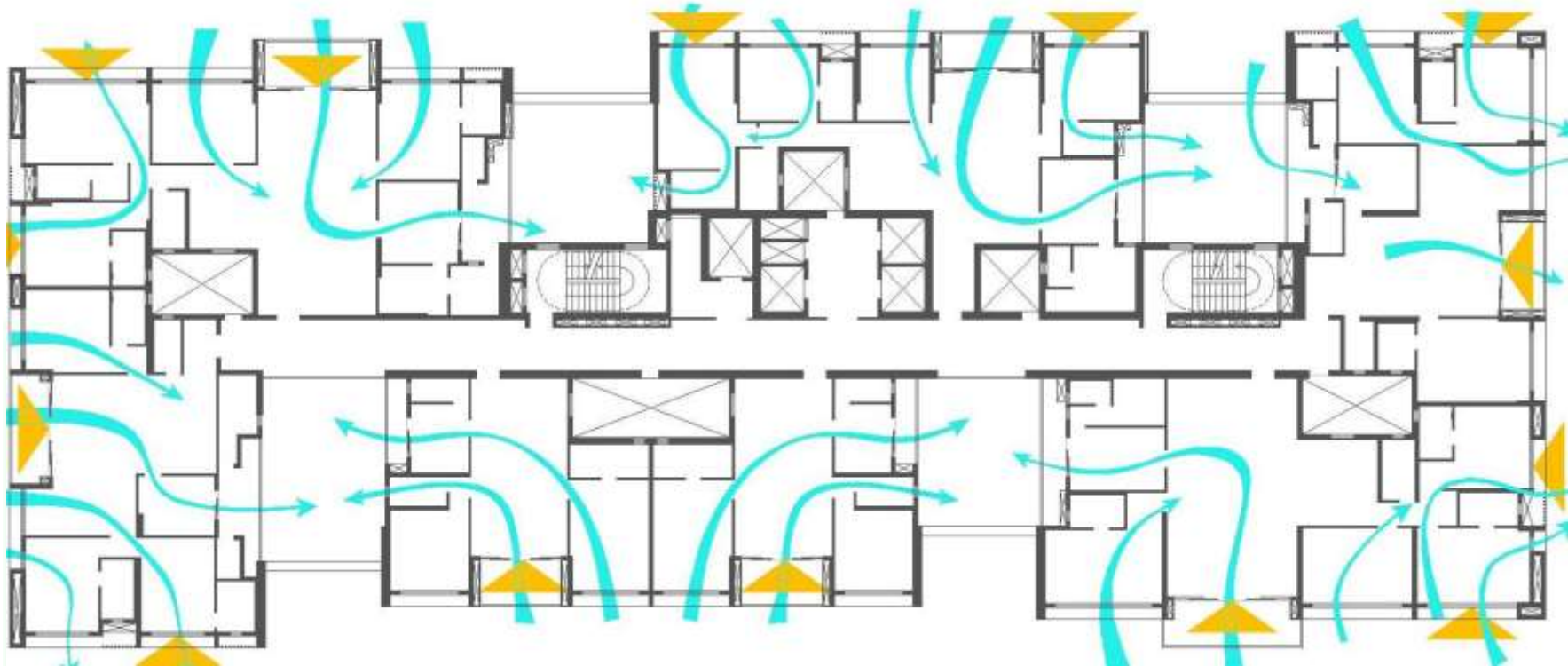
Natural ventilation wind flow diagram through typical dwelling unit
