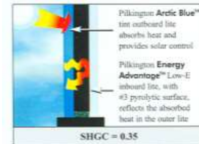
Combining the solar control properties of a tinted or reflective outboard lite (such as the Pilkington Arctic Blue™ High-Performance Tint shown here) with the thermal control properties of Pilkington Energy Advantage™ Low-E gives you an almost limitless
